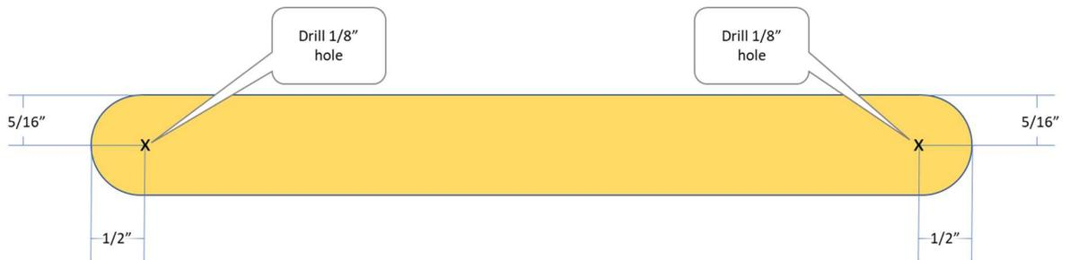
**Why we do this:** We need a place for our axels to pass through our transporter, so the wheels and axels don't fall off as the transporter moves. This is what is known as a fixed axel design and does not allow for steering to the right or the left.
